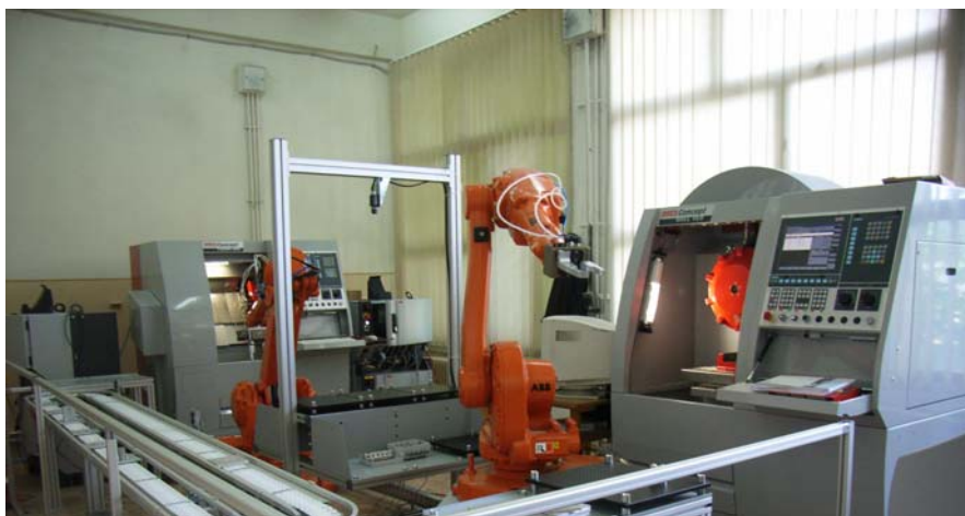
Fig.2. The Flexible manufacturing cell installed in the VEGA lab
